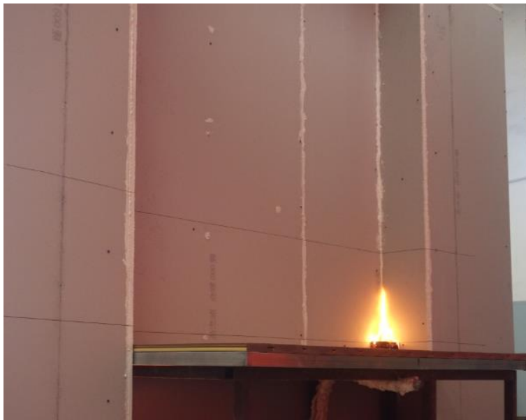
Fig. 2 Exposed Side during the radiant heat test
